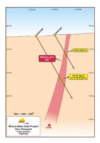
Figure 11: Emu drill hole cross section 7,038,740N
